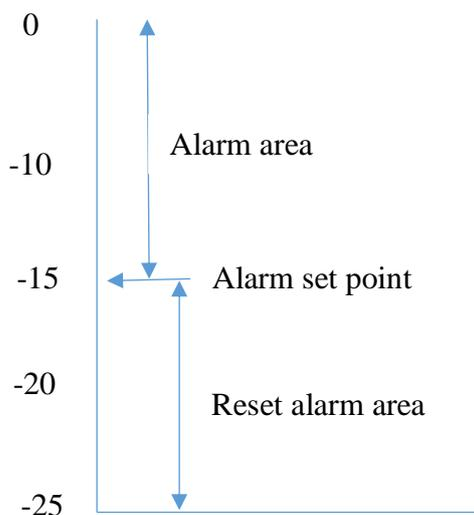
High Alarm: The unit will alarm if the current temperature is equal to or greater than the programmed high set point temperature.
