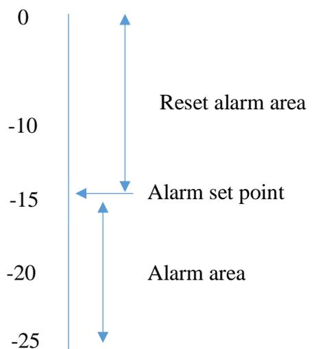
Low Alarm: The unit will alarm if the current temperature is equal to or less than the programmed low set point temperature.
